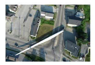
Once the potential routes have been selected, Sewall conducts field survey and works with selected trucking specialists for the wind farm, the Maine Department of Transportation (MaineDOT), and local towns and cities to develop plans for permanent or temporary modifications. Sewall develops these plans to meet MaineDOT and/or local requirements to acquire permits for the necessary work.
